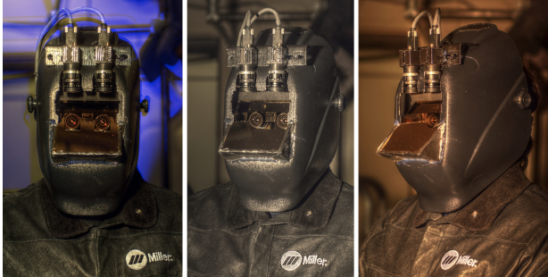
Figure 1: EyeTap welding helmet causes the eyes themselves, to, in effect, become both cameras and displays by providing exact POE (Point-of-Eye) capture for a stereo headset display.
